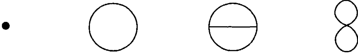
Figure 16.1. Feynman diagrams with zero, one, or two loops for the quantum effective action of the theory of a neutral scalar field \phi with interaction \phi^4 .
