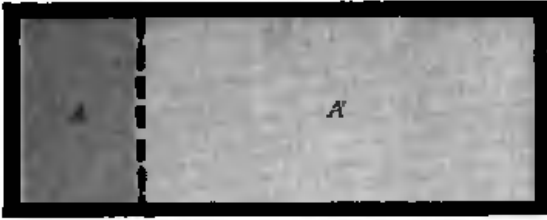
Fig. 6·9·1 A small system A separated from a much larger system A' by a perforated partition. The systems can exchange both energy and particles.
