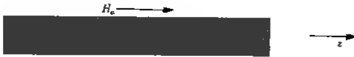
Fig. 11·1·1 A long cylindrical sample in the presence of an externally applied magnetic field H_0 . Here H = H_0 and \bar{M}_0 = \chi H .
