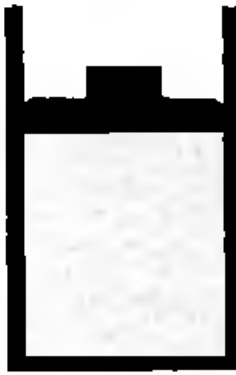
Fig. 4·4·1 Diagram illustrating specific heat measurements of a gas kept at constant volume or at constant pressure.
