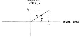
ANY C.N. THEN CAN BE REPRESENTED AS A POINT IN THE COMPLEX PLANE AND LOCATED BY THE COORDINATES OF AND B. IT IS OFTEN TIME CONVIENT TO REPRESENT THE C.N. IN POLAR COORDINATE NOTATION. If WE LET
