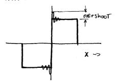
There is a way around The overshoot Difficulty And That is to attenuate the amplitude of the higher order terms. Thus Their effect is less and the Limiting behavior of the series is much smoother. We can put a factor of the fourier series and have
