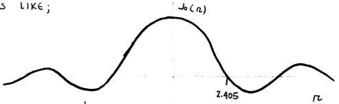
$n = \mathcal{K}_p = \rho(\omega_{j^2}^2 - K_3^2)^{\frac{1}{2}}$  if we require  $\phi = 0$  at  $\rho = 0$  Then  $J_0(Xa) = 0$  implies that  $\mathcal{K} = 2.40$  s/a. Now if  $\omega_{j'}(x) = 0$  is less. Than 2.405/a. The exponential is negative and real and the wave will Not propagate into the pipe. Dim the otherhand if the frequency is high enough, the wave Gets transmitted.
