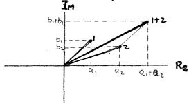
This DIAGRAM Shows THAT THE TWO C.N'S Add JUST LIKE VECTORS ACCORDING TO THE WELLKNOWN PARALLELOGRAM RULE.
