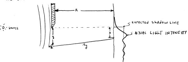
IN order to find The LIGHT INTENSITY AT A DISTANT POINT X ON A SURFACE R feet from The KNIFE WE MUST USE HUYGEN'S Principles which requires us to Add ALL The Amplitudes of The Incremental Electric fields incident on X. Thus we have That
